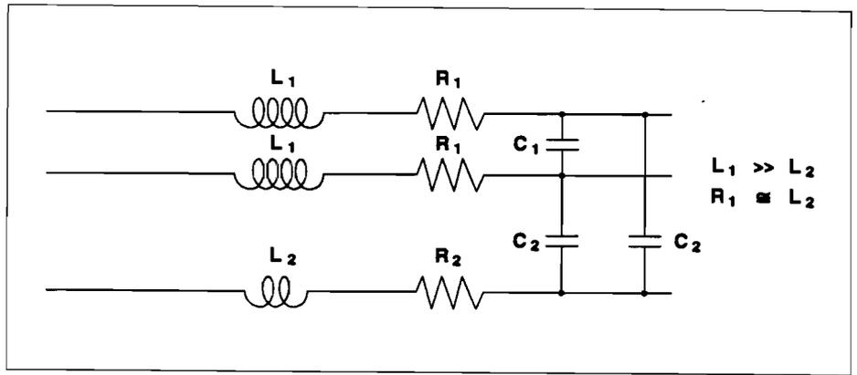
Figure 4: Three-phase scheme phase impedances
