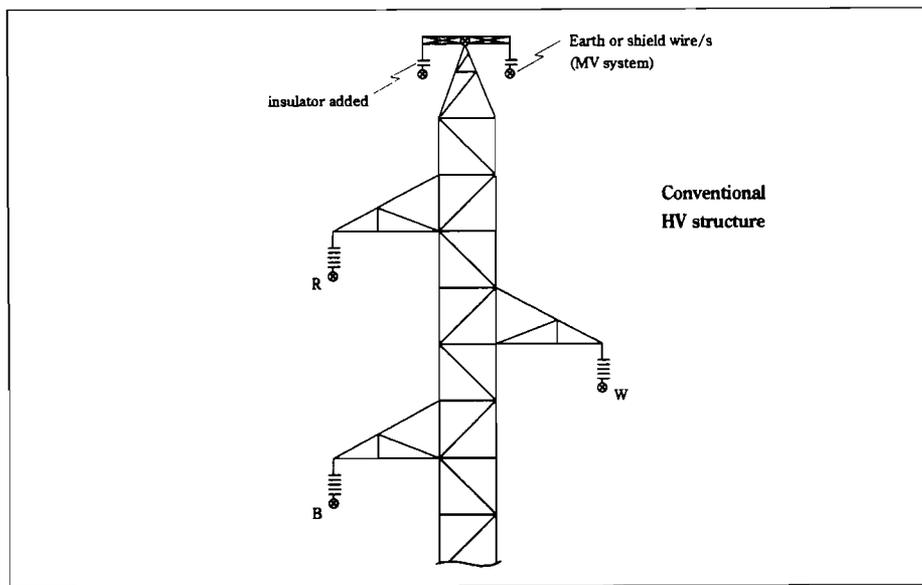
Figure 1: Typical earth wire tower configuration
