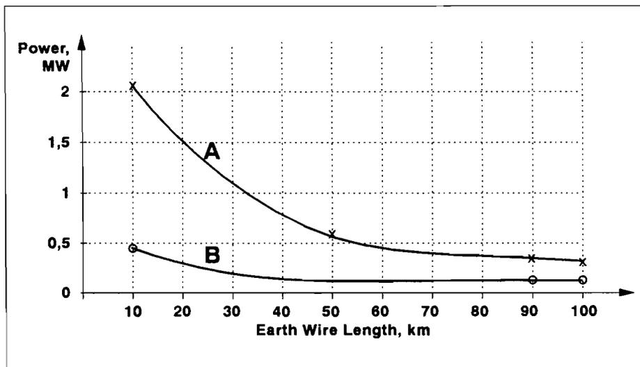
Figure 9: Power transfer capacities of earth wires
