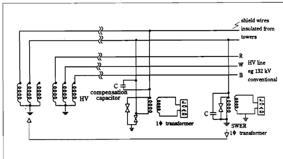
Figure 2: Single-phase (balanced) and SWER schemes
