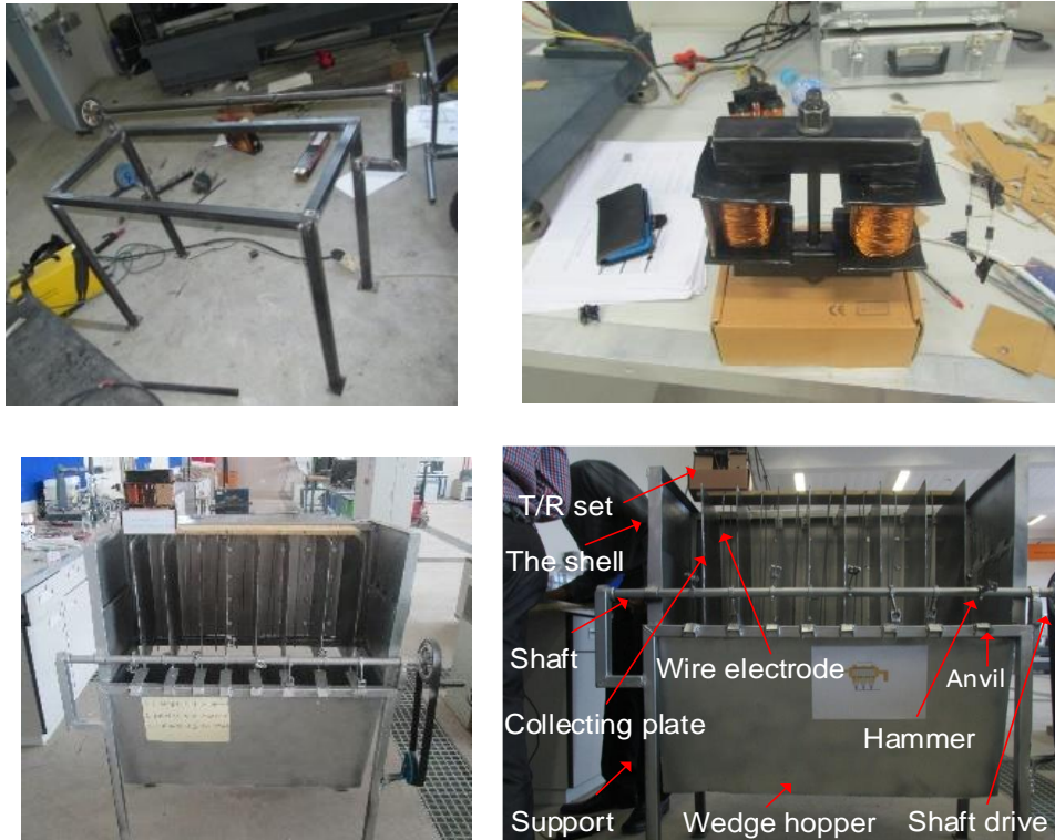
Figure 19: Construction of a mock-up ESP.
