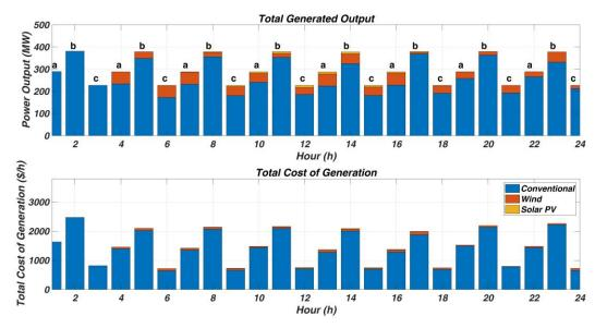
Figure 9: Integrated system output with respect to the generator schedules.
