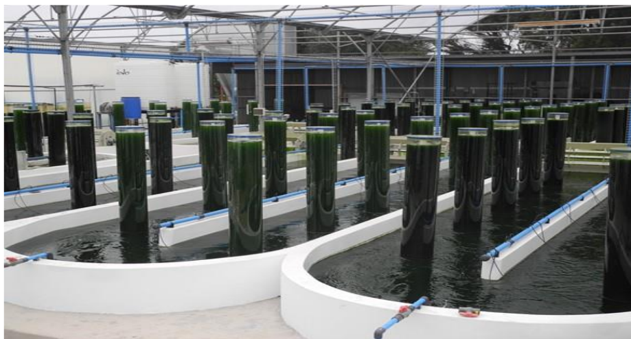
Figure 1: Production of microalgae biomass using photo-bioreactors at InnoVenton, Nelson Mandela University Port Elizabeth, Eastern Cape, South Africa.
