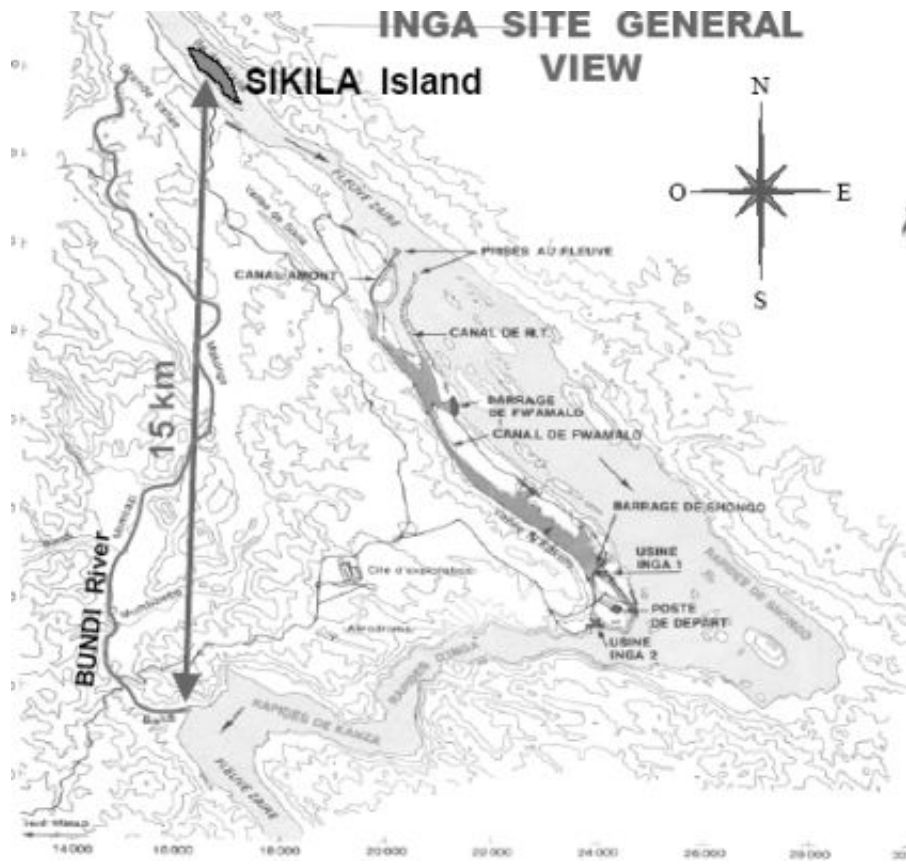
Figure 1: Inga 1 and Inga 2 and where Inga 3 and Grand Inga will be constructed
