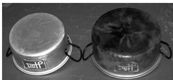
Figure 7: Pot on right blackened after boiling water once using ethanol fuel in a prototype cooker
