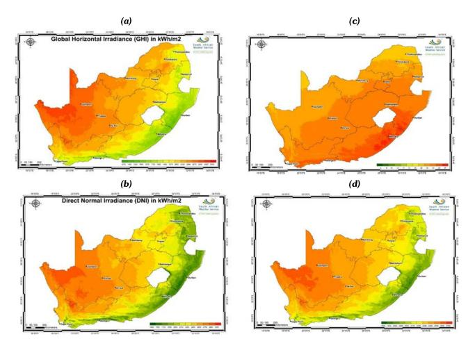
Figure 4. High resolution maps of global horizontal (a) and direct normal irradiation (b) for South Africa. Map (c) shows the local optimum inclination angle for photovoltaic installations; map (d) shows the optimally inclined plane global irradiation and PV energy yield in kWh/m<sup>2</sup>.
