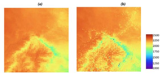
Figure 6. Global optimally inclined irradiation (kWh/m<sup>2</sup>/year) for the area bounded by 27° 30' S, 30° S, 27° 30' E, 30° E; without (a), and with (b) terrain effects.
