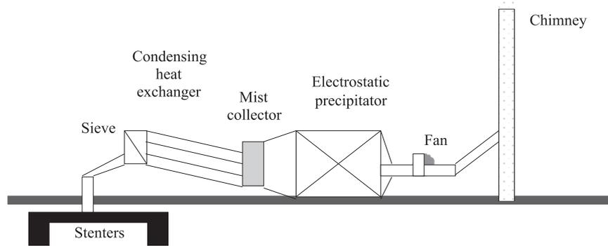
**Figure 4: Coupling heat recovery and environmental pollution control**
