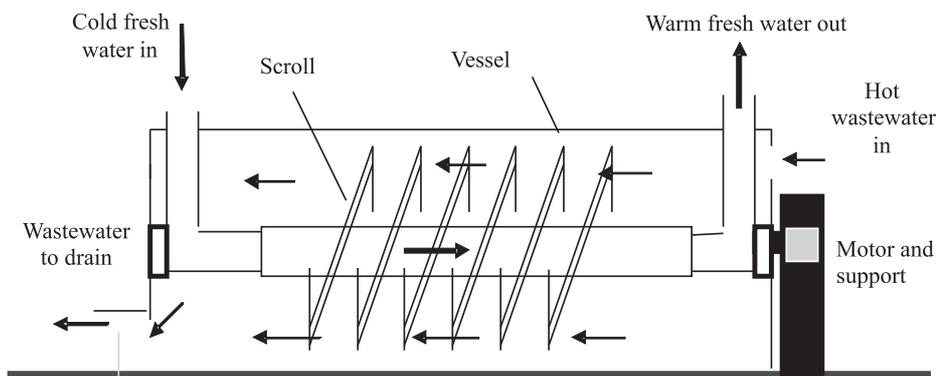
Figure 3: Spiral or rotary heat exchanger
