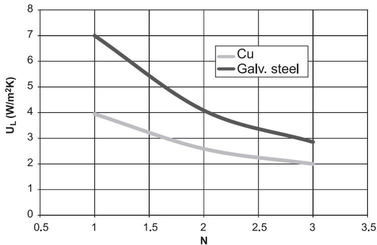
Figure 2: Variation of top-loss coefficient with number of glazing covers, N
