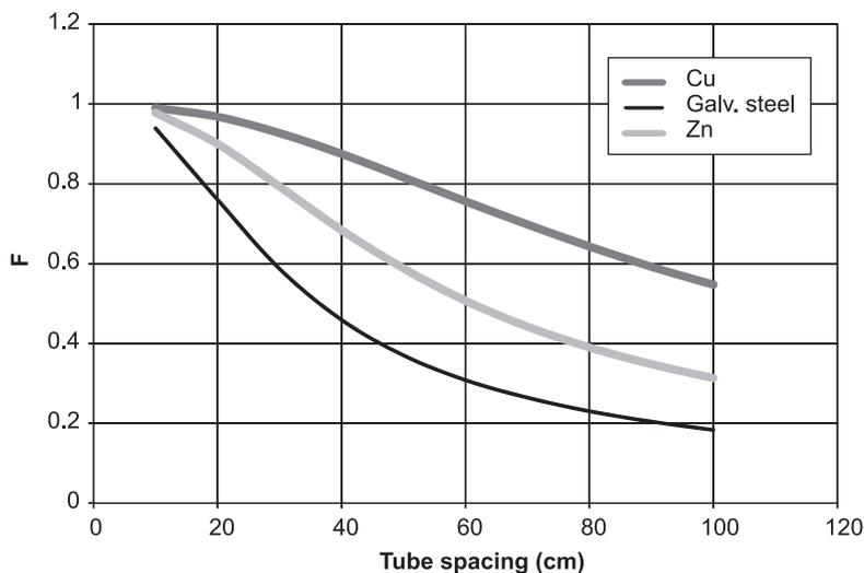
Figure 3: Fin efficiency, F against tube spacing for various absorber plate materials
