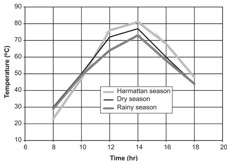
**Figure 1: Hourly temperature profile of the NCERD solar water heater for various seasons**
