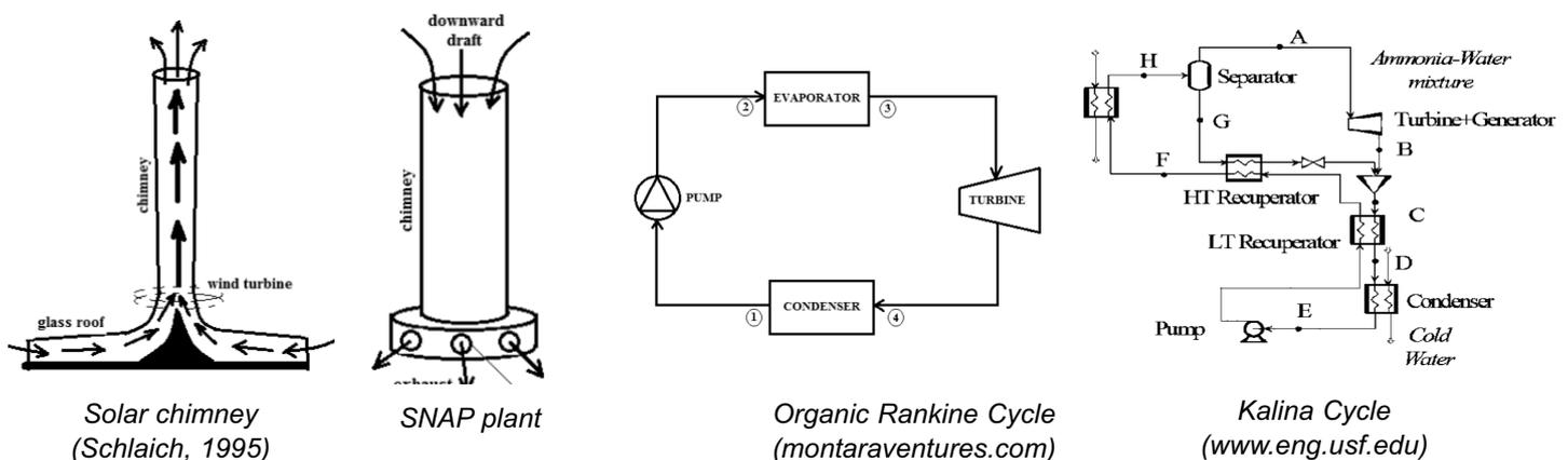
Figure 1: Examples of low temperature solar thermal energy technologies
