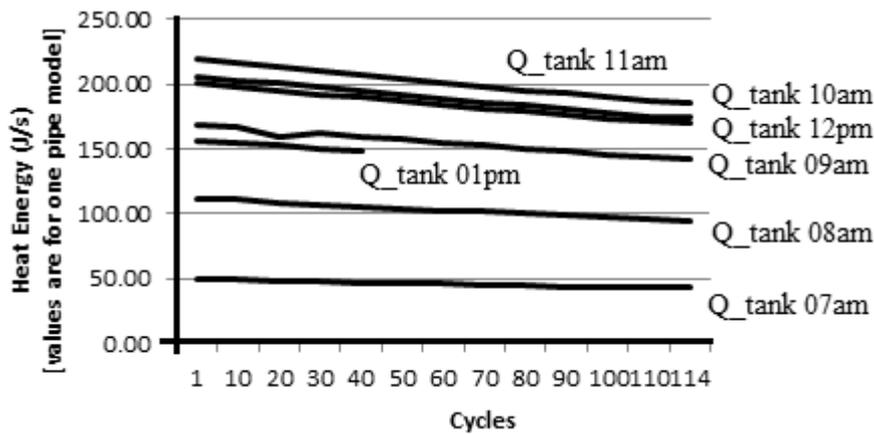
Figure 14: Heat energy rates for storage
