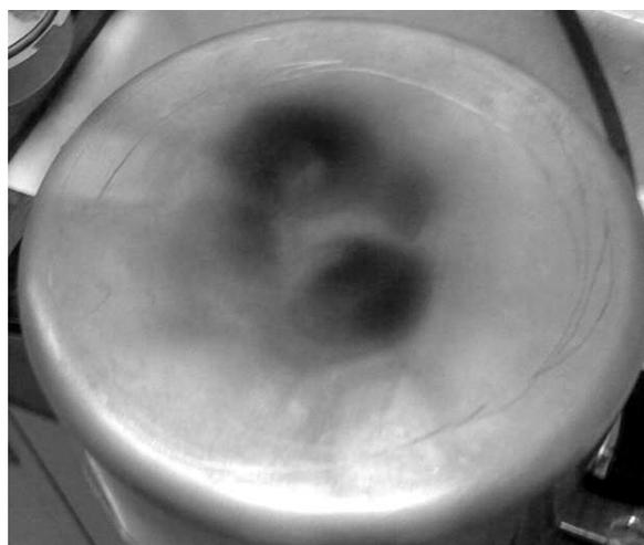
**Figure 3: Base of pot after a single cooking test**
