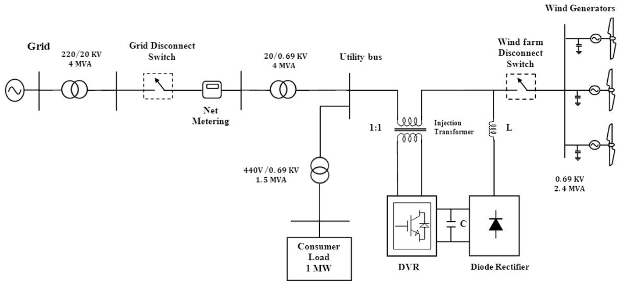
Figure 2: Grid connected FSIG with DVR protection
