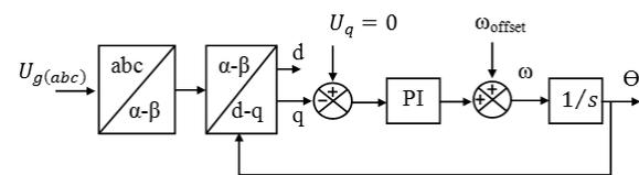
**Figure 5: Software phase locked loop circuit**
