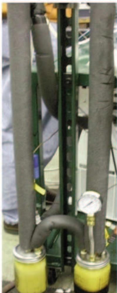
**Figure A3: Bio-oil condensers and containers**
