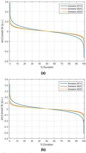
Figure 11: Duration curves of (a) day-ahead and (b) hour-ahead forecast errors.
