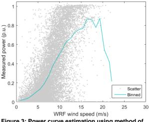
Figure 3: Power curve estimation using method of binning.
