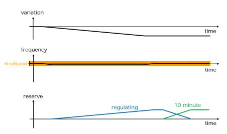
Figure 13. Illustration of the use of different reserve categories in the case of a load or wind power ramping.
