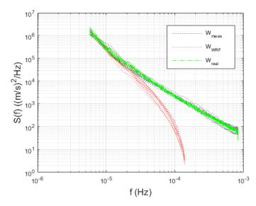
Figure 7: Power spectral densities S(f) of measured wind speeds w<sub>meas</sub>, for ten masts in South Africa and the corresponding weather model wind speeds w<sub>WRF</sub> and real time wind speeds w<sub>real</sub> simulated with CorWind.
