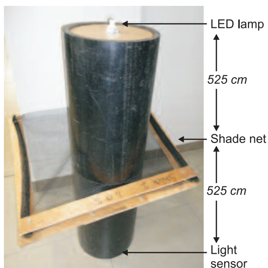
Figure 6: Practical setup for verifying the shade net specifications.
