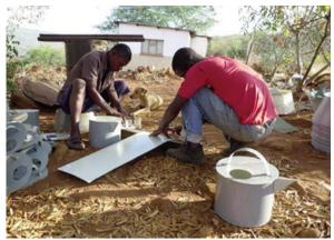
Figure 7: Local artisans manufacturing the 'Chichakuluma' kettle.
