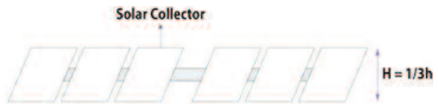
Figure 5: Planar (2D) arrangement of solar panels
