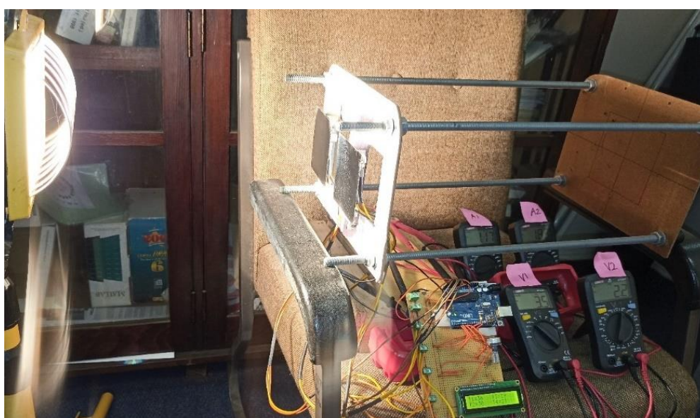
Figure 7: The thermoelectric generator system with black-coated roof sheets in closed circuit position during experiments at 600 mm.
